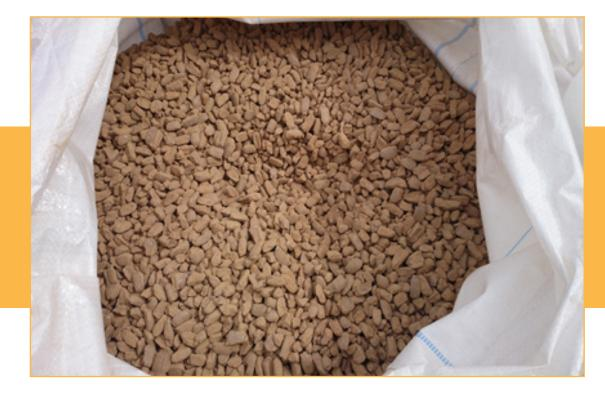
SlagMag 80 is a slag conditioner used in EAF melting furnaces for increasing MgO content in a slag. Proper MgO saturation is directly correlated to a decrease in refractory wear and the formation of foaming slag.
